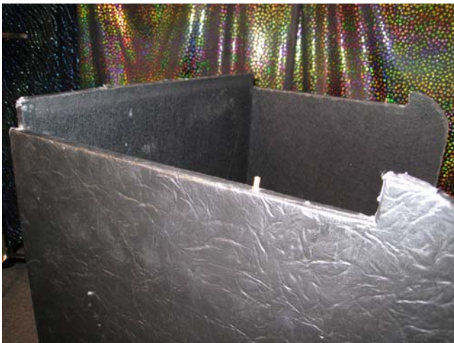
Side view with top removed – pins anchor sides to top.
